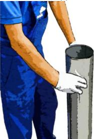
2. Prepare another pipe. Orient the second pipe with its male end pointing down.
